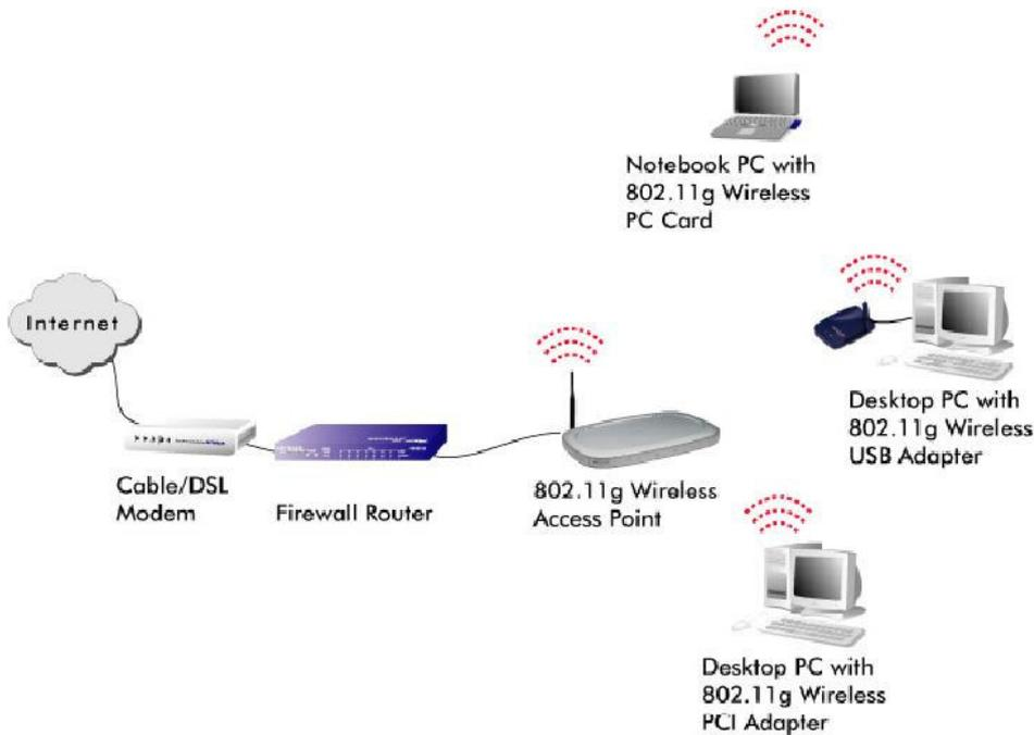
In the above picture you can see how the network works using a laptop, 2 desktop pc's and a wireless router.
